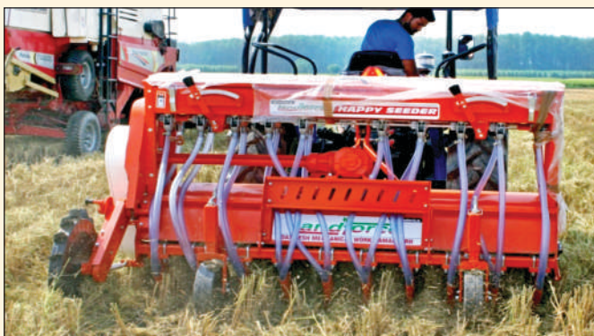
Demonstration of rice residue management through happy seeder machine
