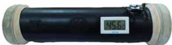
Modified artificial vagina with temperature control
