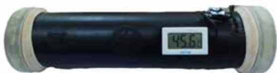
Modified artificial vagina with temperature control
